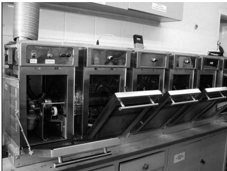
Figure 4. Continuous microwave reactor with rotating quartz tube for the synthesis of high-molecular weight epoxy resin (Ertec, Poland).
